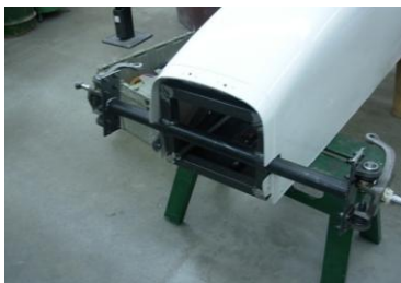
Front End Assembly on the Car
